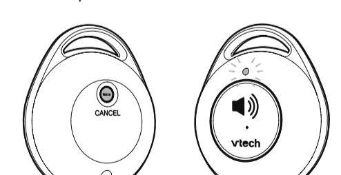
It takes up to 60 seconds to complete the registration. When the registration is successful, the red LED lights on the SOS pendant turns off, and the telephone base beeps and its visual ringer indicator light turns off.
