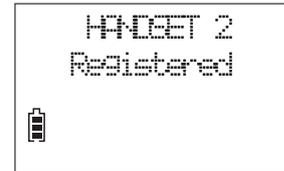
When the registration is successful, the handset displays **HANDSET X Registered**.
