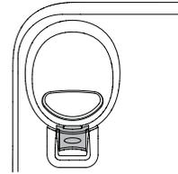
The protruding edge of the handset tab holds the corded handset in place when the telephone is mounted on the wall.
