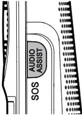
Press and hold **AUDIO ASSIST/SOS** on the cordless handset for 3 seconds. The telephone base announces, "Emergency mode is activated" and pages all registered devices. All devices ring an alert tone, and after 20 seconds, the telephone starts calling the preset SOS numbers.
