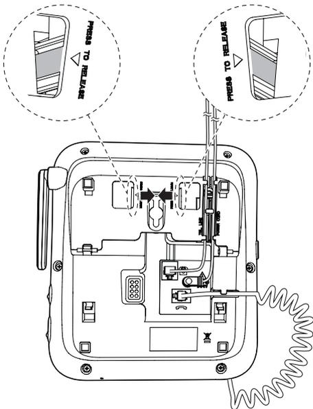
Press the tabs of the wall-mount bracket to release it from the tabletop orientation.
