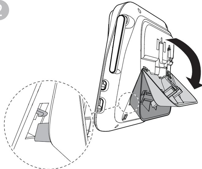
Rotate the wall-mount bracket down and push it into the telephone base until it clicks into place.
