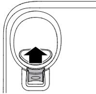
Slide the handset tab upward.
