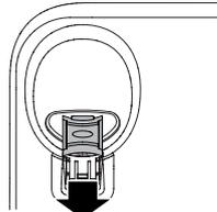
Slide the handset tab back into the slot.
