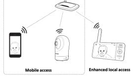
If you want to stream live video remotely with your mobile device, download and install the **MyVTech Baby 1080p** mobile app. With the mobile app, your Wi-Fi router (not included) provides Internet connectivity to your HD video monitor system. It serves as a communicating channel between your baby unit and mobile device, allowing you to monitor and/or control your baby unit wherever you are. For detail, see Download app for mobile access section in this
